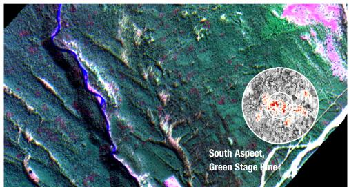
Simulated SAVI data (CASI-1500h + SASI-600) acquired near Lake Louise, Alberta. 4m resolution. Inset circle shows example of Green Stage stress in pine identified via spectral analysis of SAVI-1000 spectra. Atmospherically corrected. Displayed RGB bands: 1.48 m, 1.06 µm, 0.55 µm. Datasets acquired by ITRES. 11000 ft AGL flying helght.
