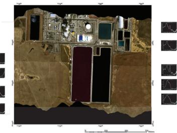
Georeferenced and radiometrically corrected microCASI airborne mosaic. Acquired March 19, 2016 over Nitrogen Production Facility, Carseland, AB. 50cm resolution: flight altitude 1000m, ground speed 75 knots. RGB Display bands: 714nm, 650nm, 550nm
